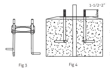
**NOTE:** Anchor bolts, template, and wire-tie bracket are attached to base plate for shipping.
